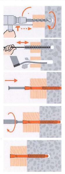
Drill the hole by **hammer drilling.**Chose drill diameter and drill hole depth according to Table B2.
