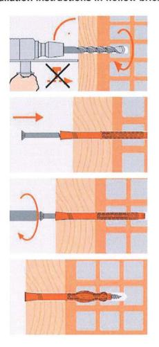
Drill the hole according to the method given in Table C6 and C7 by **rotary drilling** (without hammering) or **hammer drilling**. Chose drill hole diameter and drill hole depth according to Table B2.
