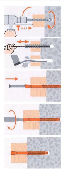
Drill the hole by **hammer drilling.**Chose drill diameter and drill hole depth according to Table B2.
